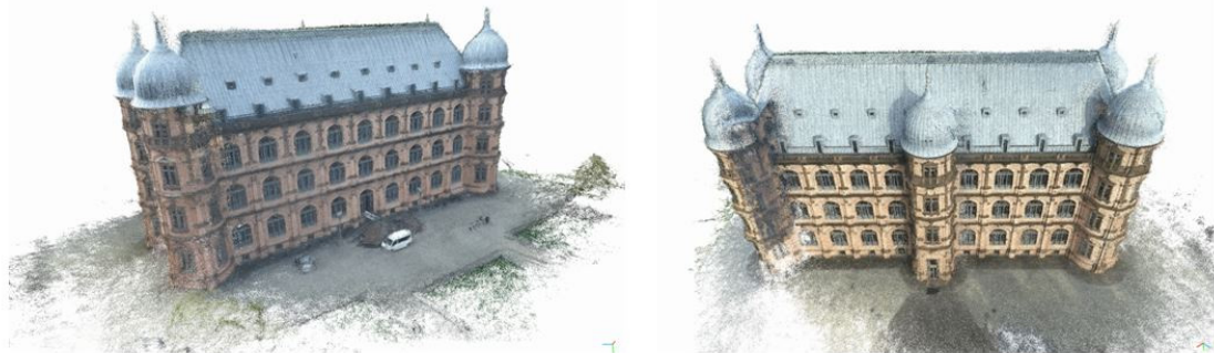
Figure 23: Reconstructed point cloud of Schloss Gottesaue. The utilized imagery was extracted from a video stream provided by Fraunhofer IOSB.
