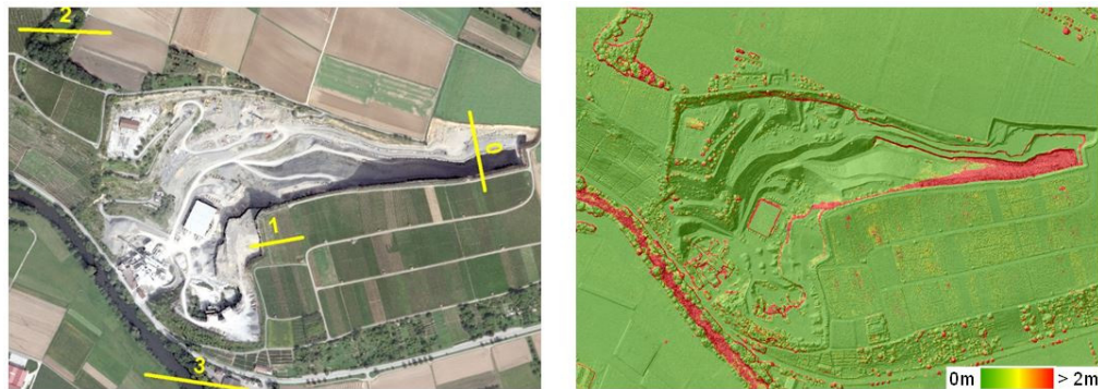
Figure 26: Ortho (left) and median DSM with RMS differences (right) for all solutions for a Vaihingen/Enz subsection.
