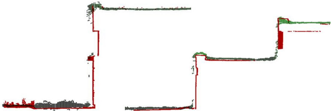
Figure 20: Comparing of the 3D point cloud from airborne images derived from dense surface matching to a terrestrial point cloud from terrestrial laser scanning. The building walls from terrestrial scanning are clearly seen in the given profile. The airborne DSM nicely fits the roof shape of the building.
