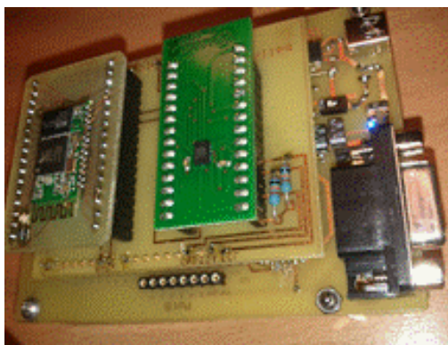
Figure 5 INS microcontroller evaluation board with BOSCH BMI055 and Bluetooth module
