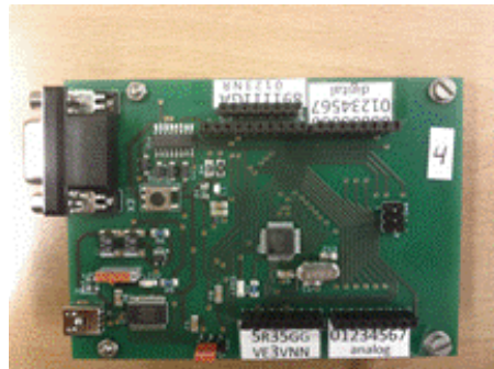
Figure 4 INS microcontroller evaluation board.
