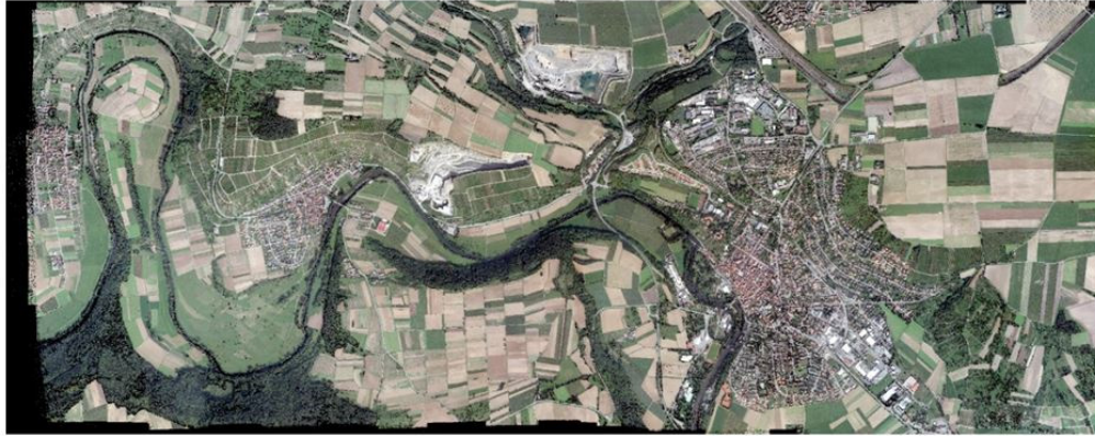
Figure 25: Vaihingen/Enz block, orthophoto, GSD is 20cm.
