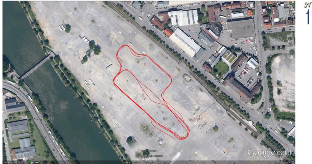
Fig. 18: Surveying layout for second kinematic track, Wasen Region © Google Eart
