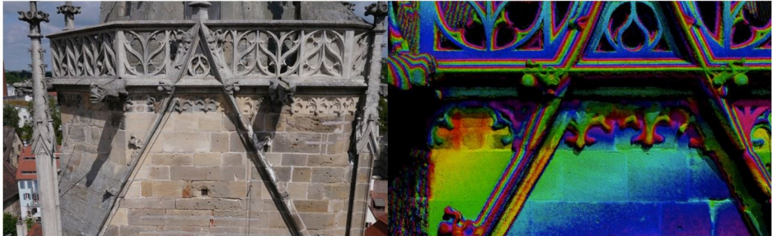
Figure 4: Depth estimation by dense image matching for a church tower in Rottenburg/Neckar, Germany. An unmanned aerial vehicle (UAS) was used to acquire multiple views of the façade. Left: image, right: point cloud from dense image matching with depth coded coloring.
