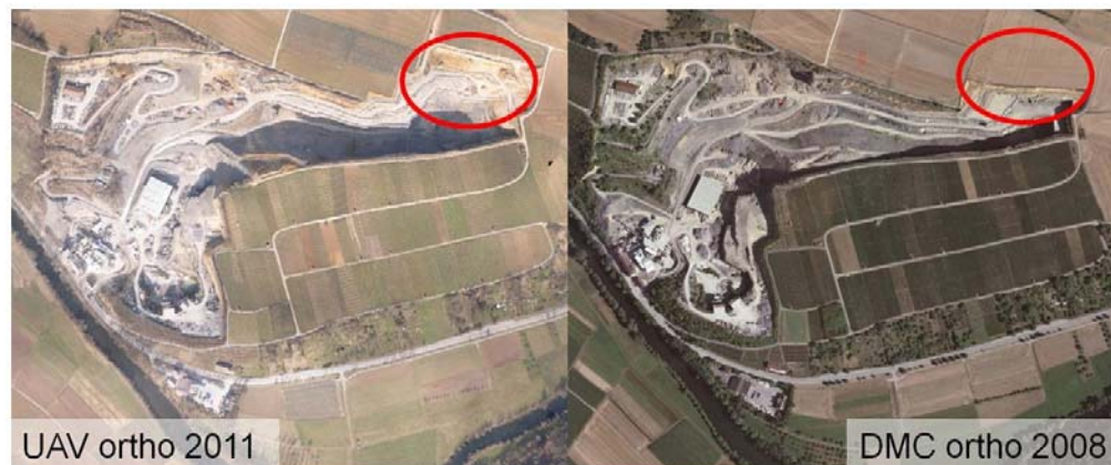
Figure 21: Orthophoto from UAV imagery (March 2011) compared to orthophoto from large format high end digital airborne mapping camera DMC (Z/I-Imaging).
