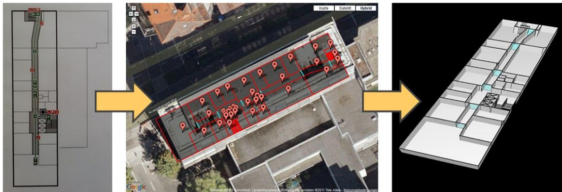
Figure 5: Evacuation plan of our institute; automatically derived 2D model in Google Maps; automatically derived 3D model with identified doors.
