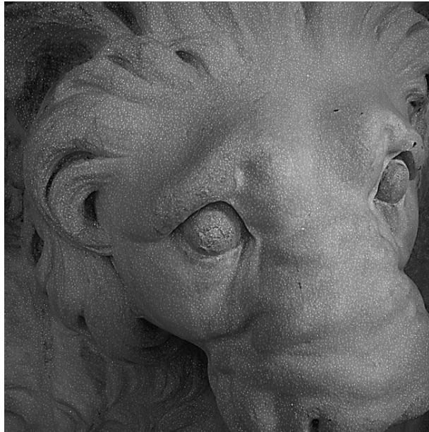
Figure 9: Image taken by one of the matching cameras. The white speckles covering the lion head's surface are produced by the Kinect's IR laser projector and are not visible to the bundle camera. The image has been slightly enhanced to make the pattern easier to see for the reader.
