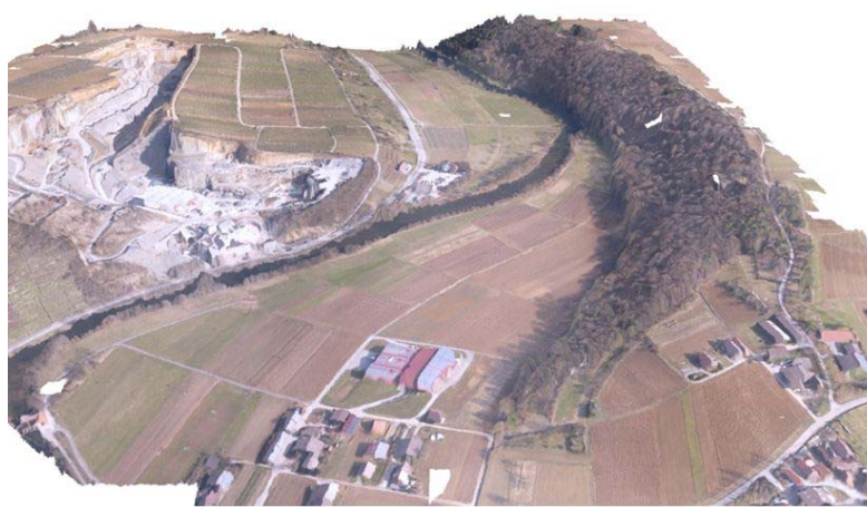
Figure 20: Quarry nearby Vaihingen/Enz: Orthophoto from UAV flight 2011, draped on the 3D surface model dense matching of UAV imagery.
