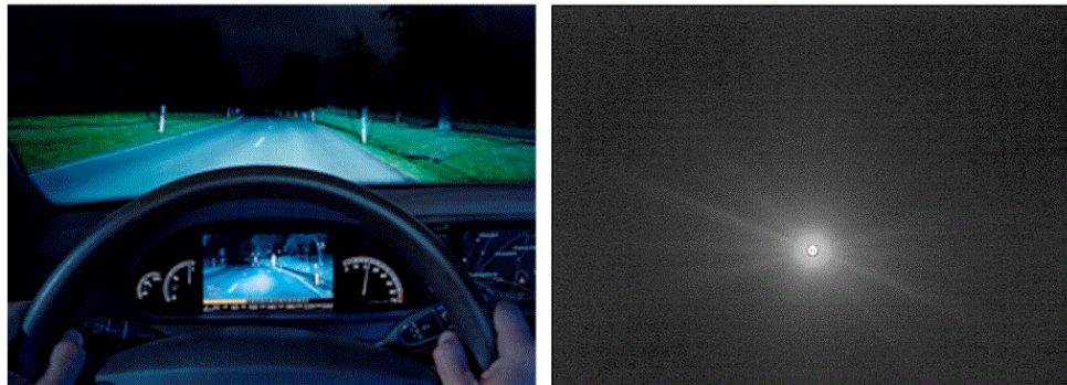
Figure 25: Night vision system (left) and stray light artefact in form of radial beams (right).
