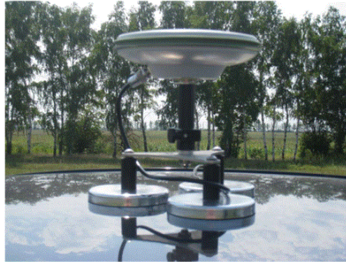
Fig. 6: Antenna (LEICA GX 1230) on the roof of a passenger car (Source of the figure: Report „Messung von GPS Tracks in Russland“ from GCI)
