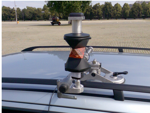
Fig. 10: Installed ublox receiver and 360° prism
