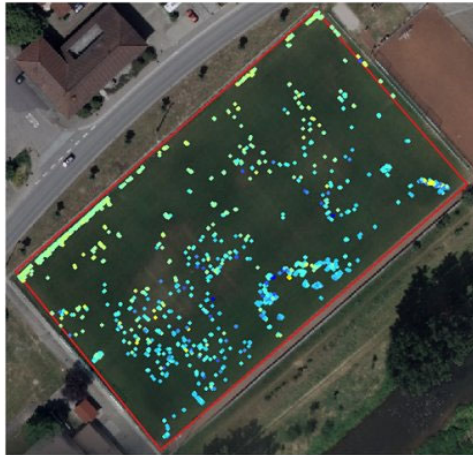
Point cloud from RMK-Top (GSD 8cm)
