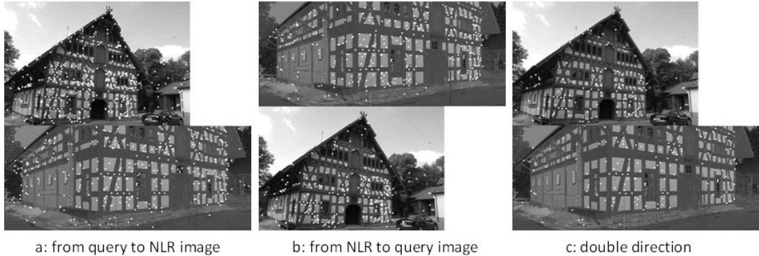
Figure 10: SIFT matching points for normalized laser reflectance (NLR) image and query image
