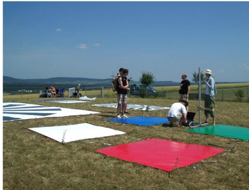
Figure 8: Ground teams performing reference measurements in radiometric test field
