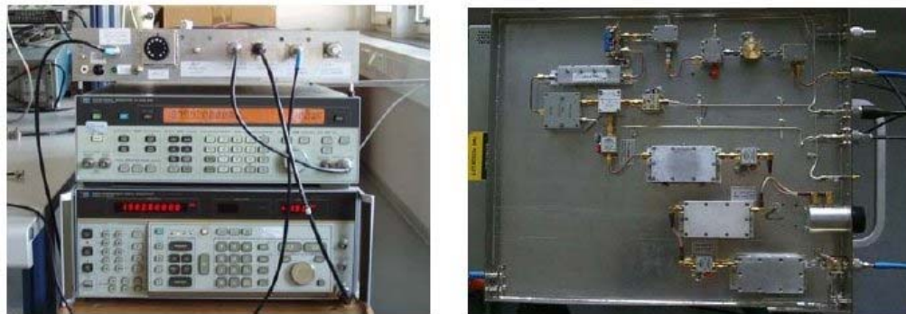
Figure 1: Modular RF front for acquiring real-time data of GPS/GNSS signals - front end with 2 local Oscillator (left) and Modular Components right
