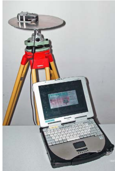
Fig. 2: Garmin eTrex Vista, adapter, shielding and laptop
