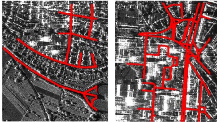
Fig. 13: Result of automated matching between the GDF-street data and SAR image.
