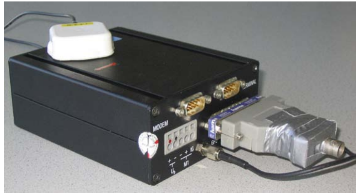
Fig. 3: Hybrid positioning system with GPS-antenna and adapter for the speed signal of the vehicle
