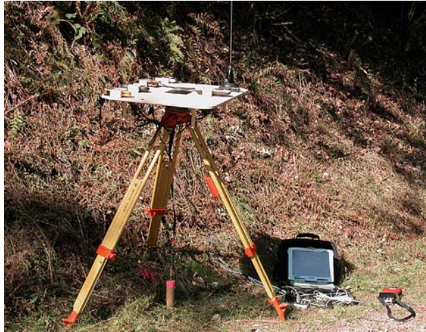
Fig. 2: Configuration for simultaneous measurements of all receivers
