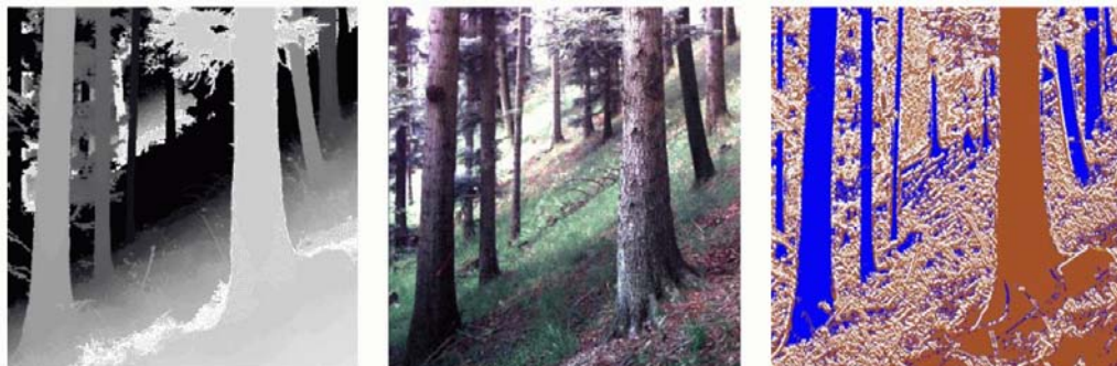
Fig. 17: Section of range image (left), coregistrated panoramic image (middle) and result of combined segmentation (right).
