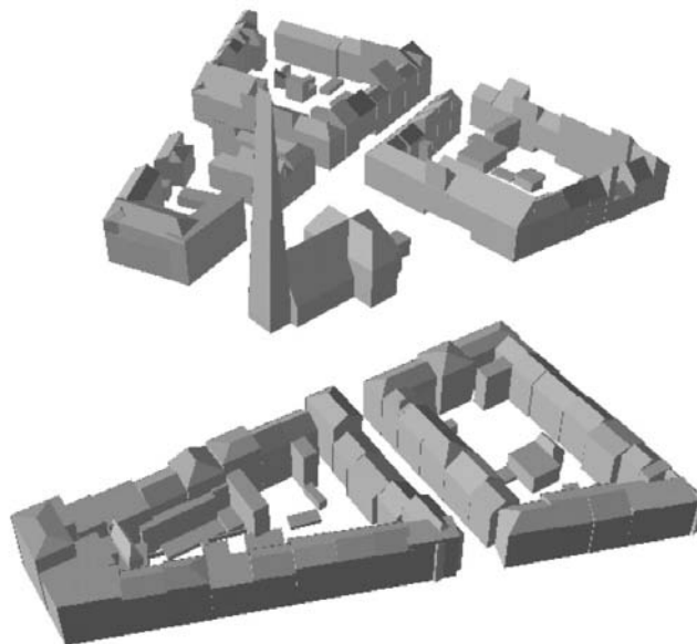
Fig. 18: Available 3D city model used as input for SAR simulator.
