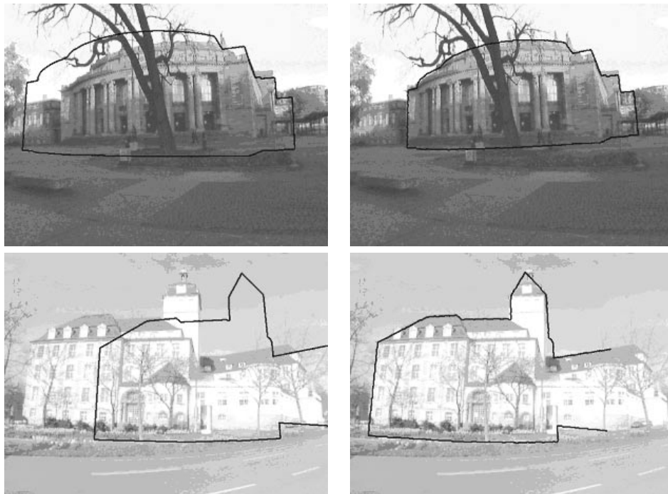
Fig. 18: CAD model of a building rendered for a given exterior orientation and the extracted silhouette to the right.
