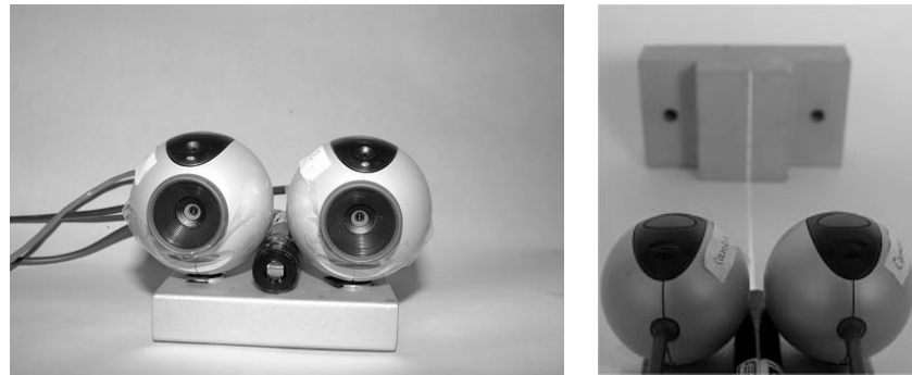
Fig. 19: (a) Laser triangulation sensor built from two web cameras. (b) The sensor and the visible laser beam on a test object.
