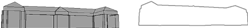
Fig. 17: CAD model of a building rendered for a given exterior orientation and the extracted silhouette to the right.
