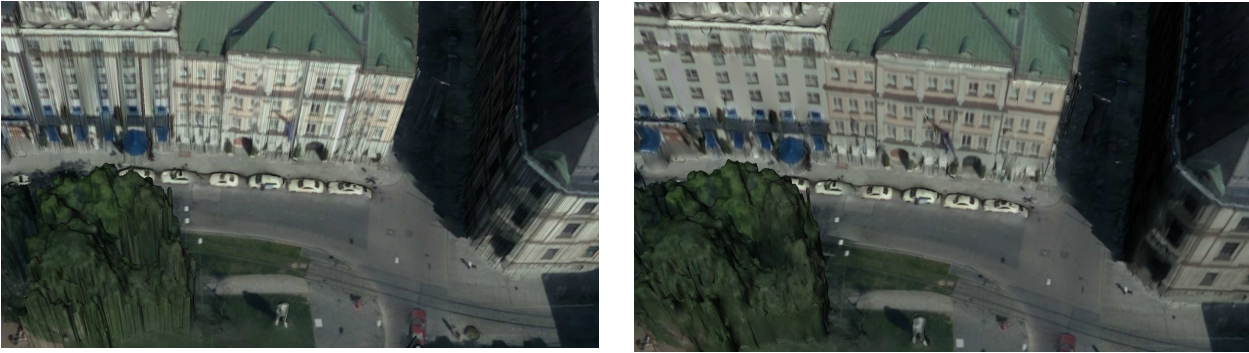
Figure 5.14: Left: Textured mesh without facade re-meshing. Right: Textured mesh with re-meshing.
