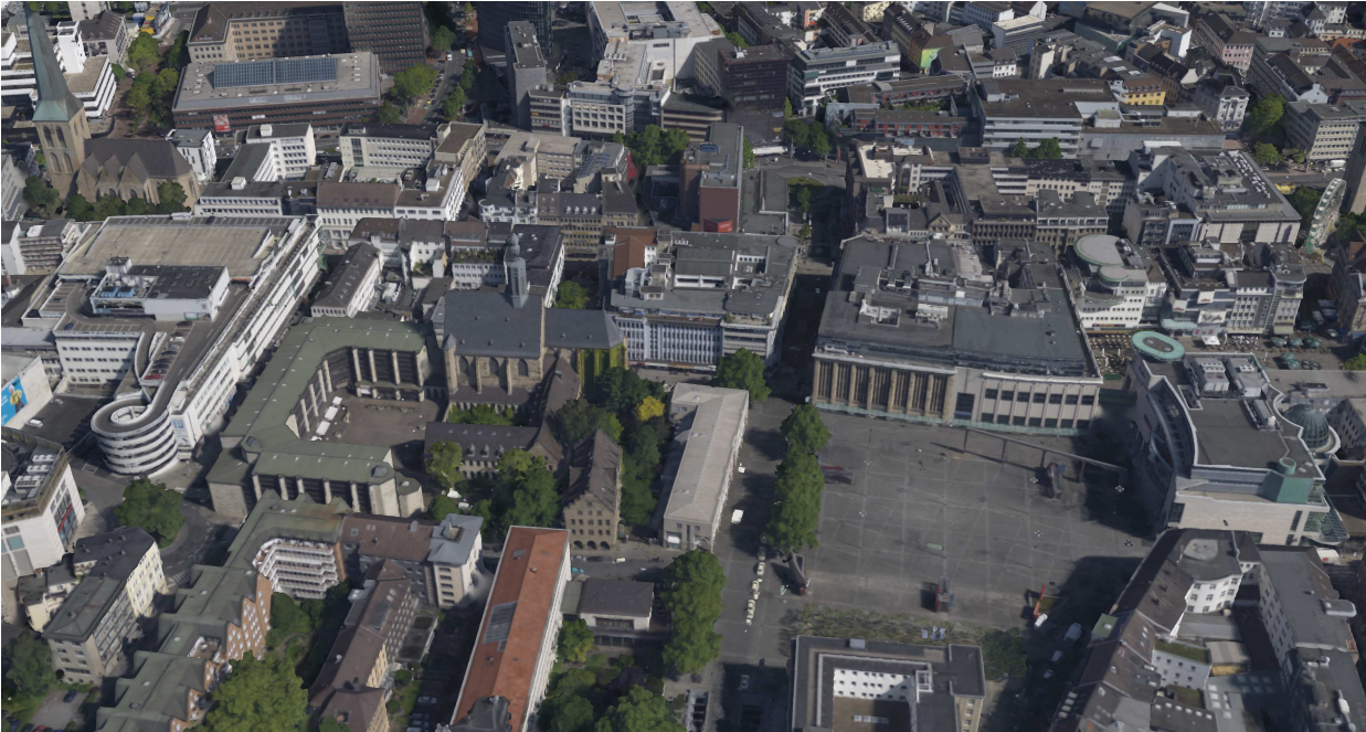
Figure 6.11: Textured mesh generated by the the proposed approach for the Dortmund dataset (14cm avg. GSD). Note that no effects of tiled processing are observable.
