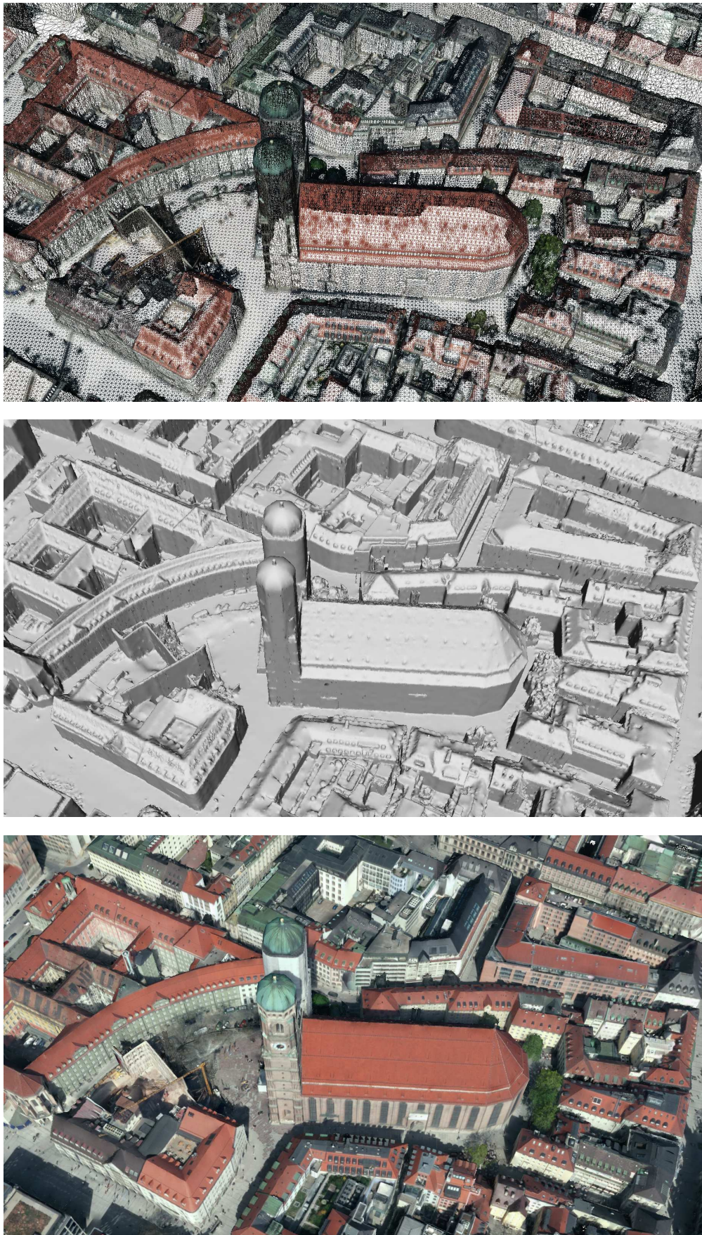
Figure 5.15: Top: Mesh generated by the RQT approach including facade re-meshing. Middle: Shaded visualization. Bottom: Textured mesh.
