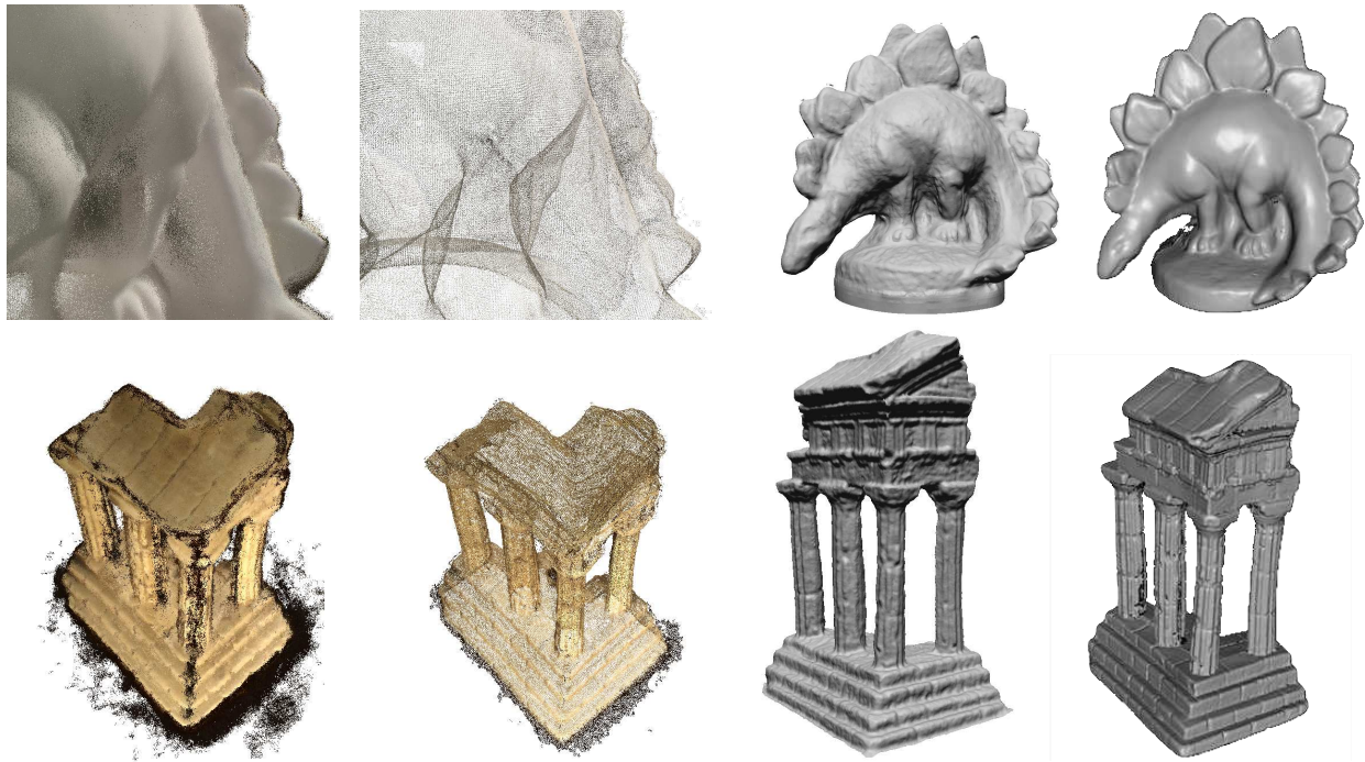
Figure 6.8: Results for the temple and dino data sets. From Left to right: raw point cloud; oriented points resulting from the our method; mesh generated by Poisson reconstruction using our oriented points; ground-truth mesh.
