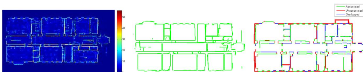
Figure 4.9 – 2D floor plan from point density histogram. From left to right: 2D point density histogram, estimated Hough lines and overly with ground truth (labeling based on detected lines): green and blue line segments are modeled by the algorithm, while red segments are missed. (adapted from Okorn et al. (2010))
