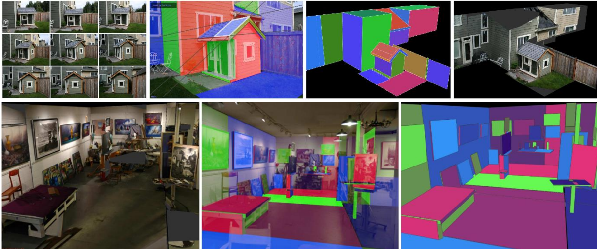
Figure 4.3 – An interactive system interface for generating 3D photorealistic models from unordered photographs. Top (from left to right): input photographs, 2D sketching of polygons, geometric model and textured model. Bottom (example in an indoor scene, from left to right): input photograph, overlay of the model on the photo and geometric model. (from Sinha et al. (2008))
