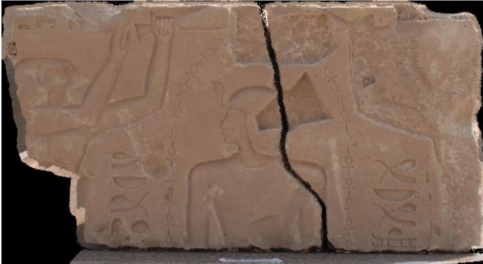
Fig. 7.14. Re-colored laser scanner point clouds from 3 scans acquired by the C10 scanner of the carved stone dataset using 4 registered camera images.
