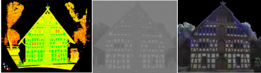
Fig.3.1. The old farm house dataset, from the left, 3D laser scanner point cloud acquired by the Leica ScanStation HDS3000 at an approximate sampling distance of 2cm, generated Reflectance and RGB images using image matrix.
