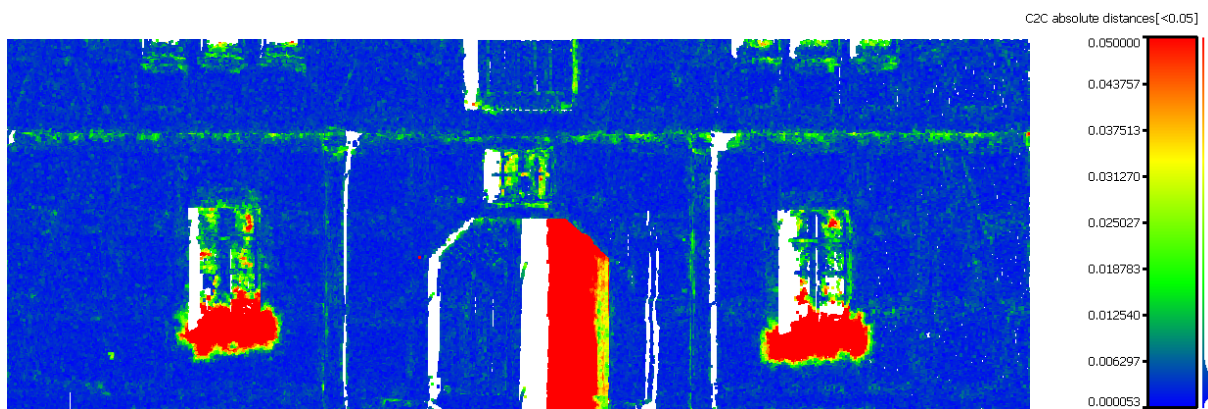
Fig.4.22. Comparison of point clouds resulted from dense image matching using the software SURE with 35 camera images and that derived by laser scanner with one scan station, in the overlap area of the old farm dataset. It shows the distance error map and the corresponding scale bar of the absolute difference distances \leq 5 cm.
