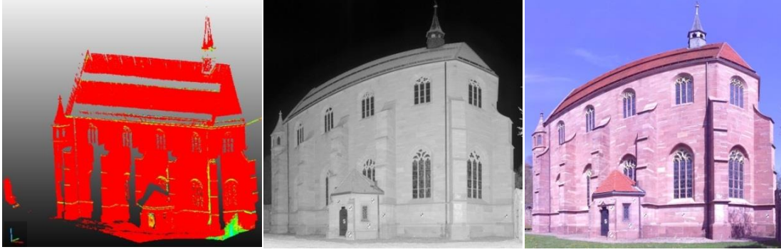
Fig.3.2. The Lady Chapel dataset, from the left, 3D laser scanner point clouds acquired by the Faro® Laser Scanner Focus 3D at an approximate sampling distance of about 7 mm@10m distance, delivered Reflectance and RGB images.
