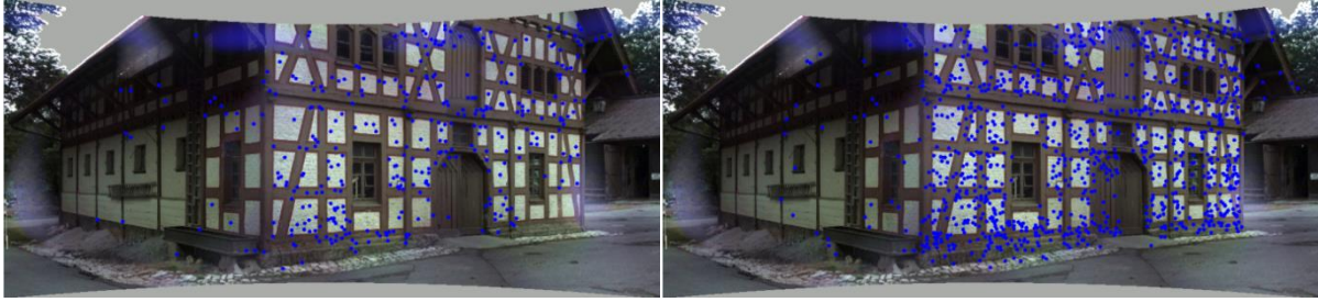
Fig. 4.18. 3D-to-3D filtered correspondences (383 keypoints) between sparse point clouds and a laser scan of the old farm house dataset using only the features appeared in the corresponding RGB image (left). 3D-to-3D filtered correspondences (1064 keypoints) between sparse point clouds and a laser scan of the old farm house dataset using all projected sparse point clouds onto the corresponding RGB image (right).
