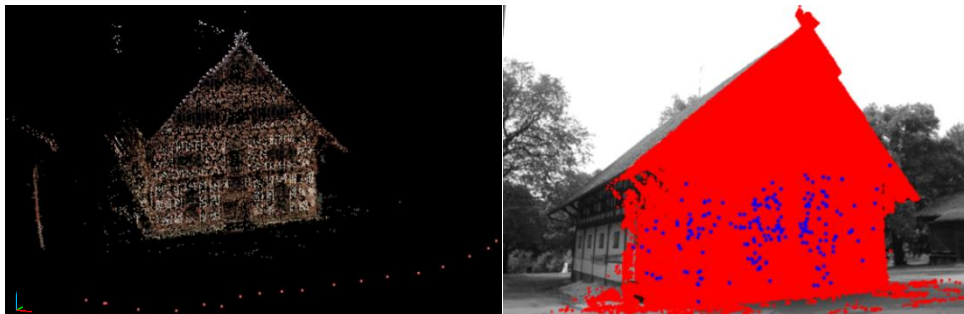
Fig. 4.12. SfM output: sparse point clouds (colored), 19 camera positions (red dots) of the old farm house dataset (left). Reprojected dense image point clouds onto a camera image (red dots) and the resulted 3D correspondences (210 keypoints, blue dots) between the latter and the laser point clouds which are used for the calculation of the seven- parameters, depicted on the camera image (right).
