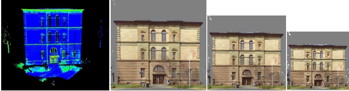
Fig.3.6. Dataset of Stuttgart University building, from the left, 3D laser scanner point cloud acquired by the Faro® Laser Scanner Focus 3D and generated RGB images with different pixel footprints; interval distance in object space (2, 5 and 9cm).
