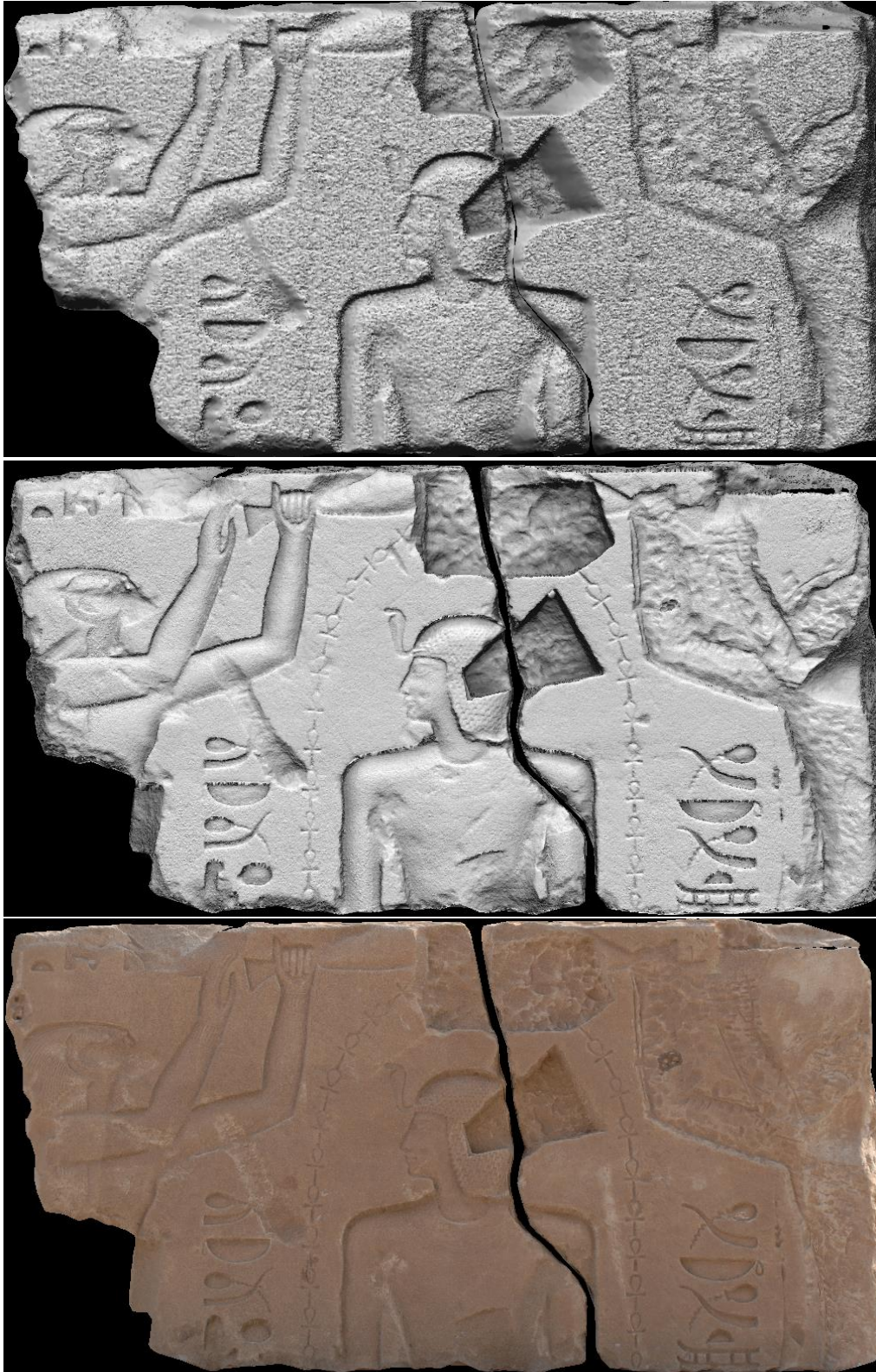
Fig.7.12. 3D triangulated models of the carved stone dataset. 3D triangulated model using the laser scanner point clouds from 3 scans acquired at an approximate sampling distance of about 2 mm by the Leica ScanStation C10 of about 1.4 Mio. (1 st row). 3D triangulated model using the dense image point clouds derived by the software SURE from direct registered imagery with subsampled set of around 5.5 Mio. points, illustrated without/with texture information respectively (2 nd and 3 rd rows).
