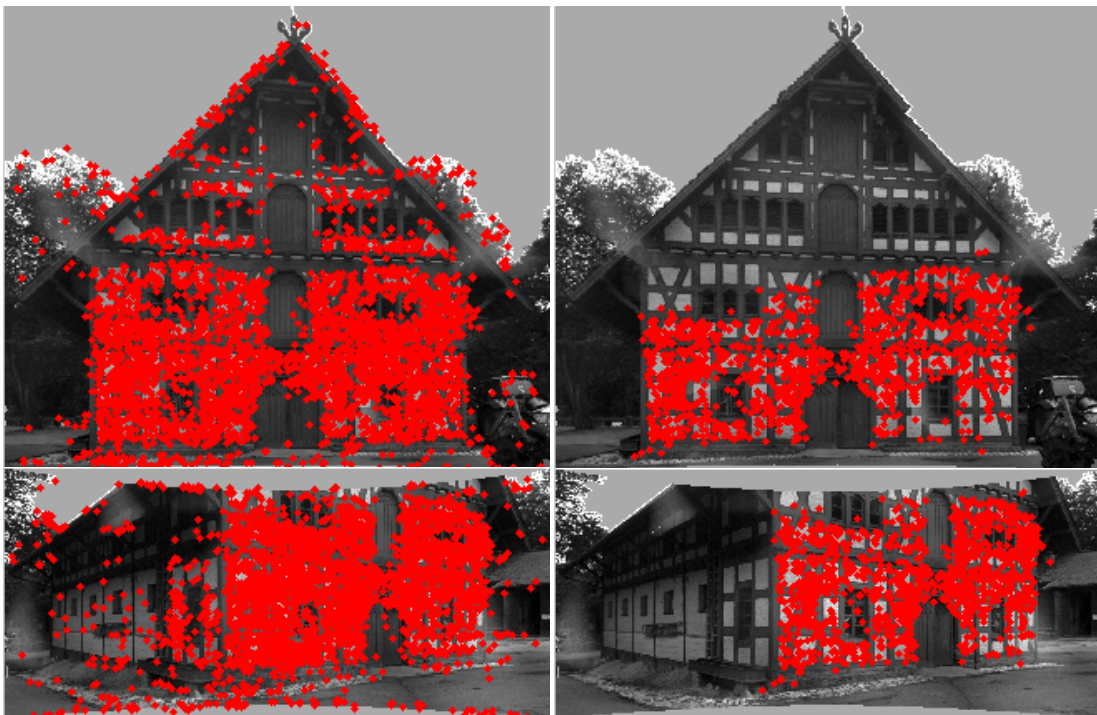
Fig.5.3. Old farm house dataset, removal of false correspondences. Correspondences (red dots), between a scan pair depicted on the corresponding generated RGB images, matched by the kd-tree descriptor comparison procedure with 4124 keypoints (left) and then filtered by RANSAC based on a closed-form space resection to obtain 1563 keypoints (right).
