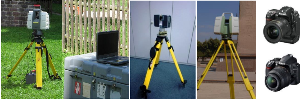
Fig.7.3. The applied sensors, (From left to right) the Leica ScanStation HDS 3000, the Faro® Laser Scanner Focus 3D , the Leica ScanStation C10, the NIKON D2X, 12 Mpx with 20 mm focal length (above) and the NIKON D3100, 14.2 Mpx with 24 mm focal length (bottom).
