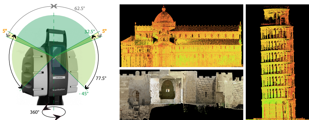
Figure 2.5: Field of view of the laser scanner HDS3000 (left) and examples of point clouds acquired with it (right). The point clouds represent two views of Piazza del Duomo in Pisa (color scale) and the fortified gate of Bab al-Barqiyya in Cairo (from the CyArk [2011] archive).
