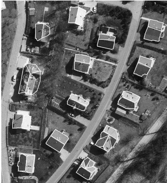
Figure A.1: Reconstructed coarse buildings overlaid on the corresponding aerial image
