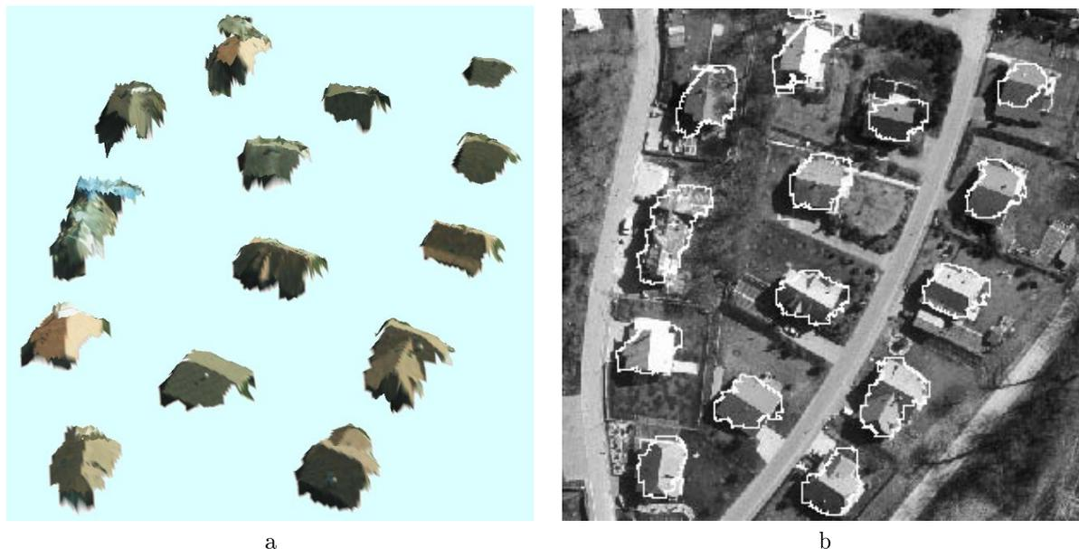
Figure 4.5: Extracted regions of interest: a) the 3D perspective of the extracted region wrapped over corresponding DSM, b) extracted region overlaid on the corresponding aerial image.
