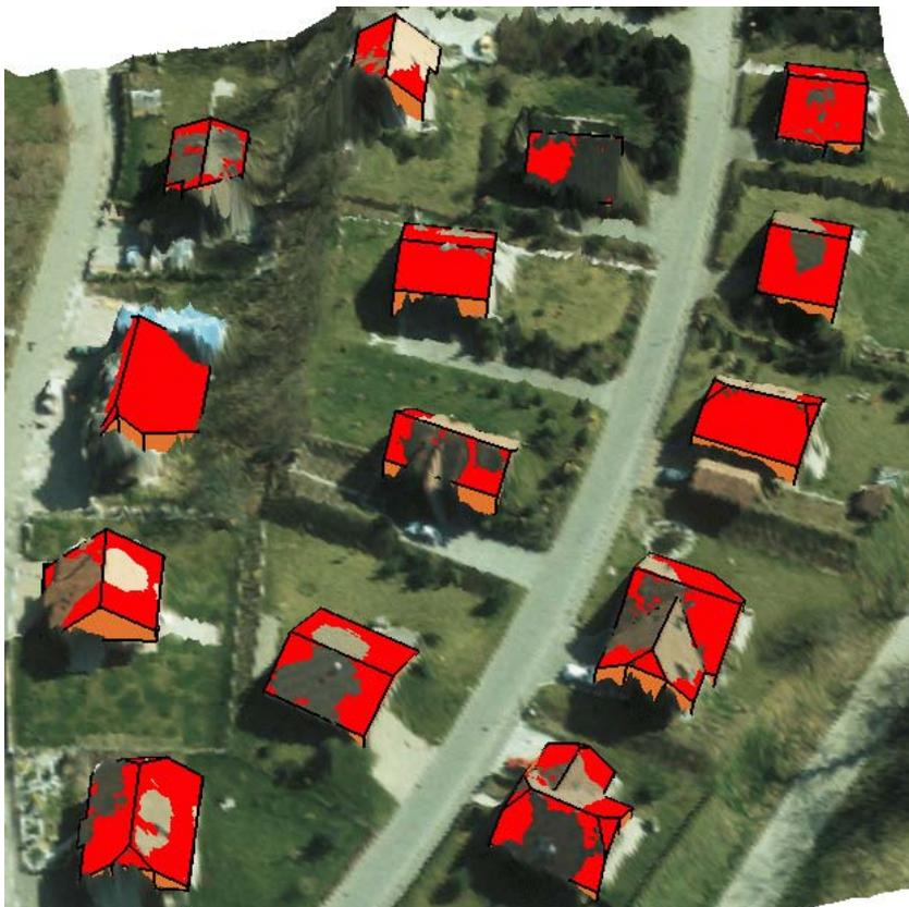
Figure A.6: Perspective view of the final 3D reconstructed buildings overlaid on the DSM
