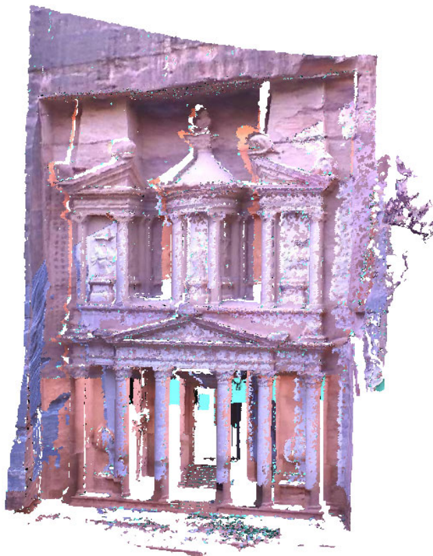
Figure 3.20: 3D textured model of the treasury using the integrated camera (3 scans)
