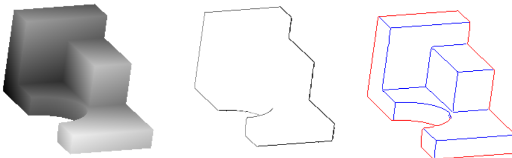
Figure 4.3: Curve block range image (OSU). Mid image shows segmentation result using canny operator. The right image shows the types of edges in the range image; crease edges (blue) and step edges (red).
