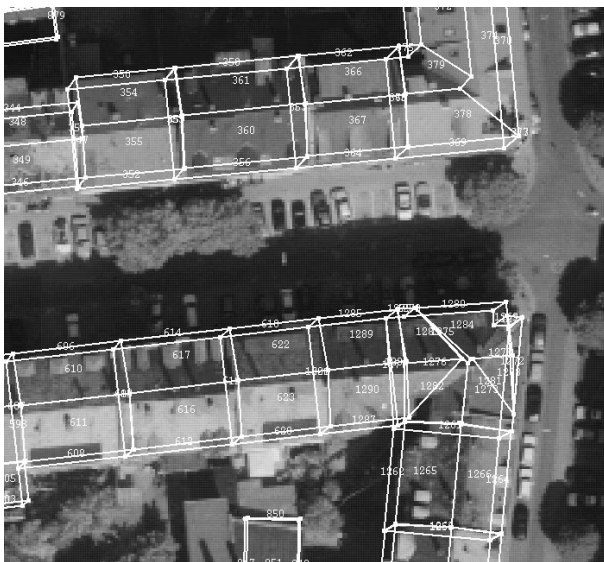
Figure 15: Reconstructed buildings projected into stereo image.
