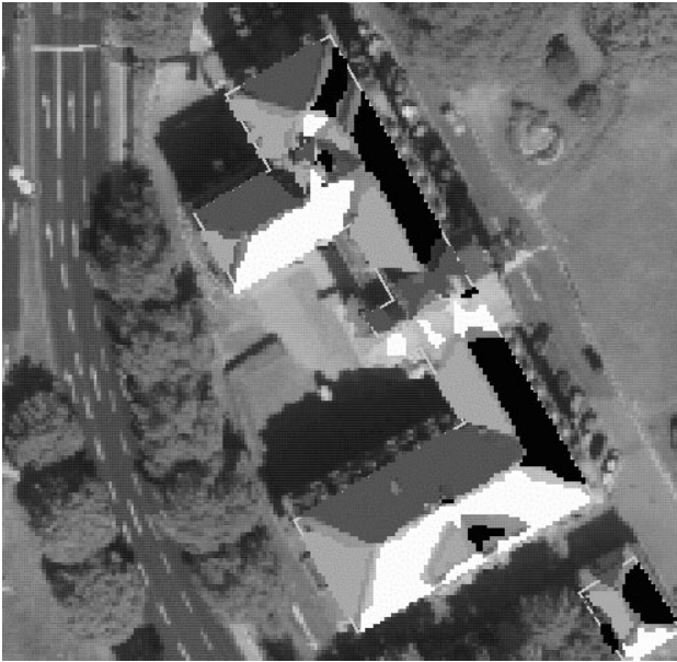
Figure 5: Segmented roof regions.
