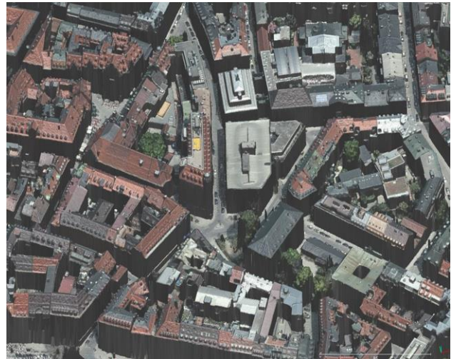
Fig. 2. Textured DSM using dense image matching for highly overlapping standard aerial imagery.
