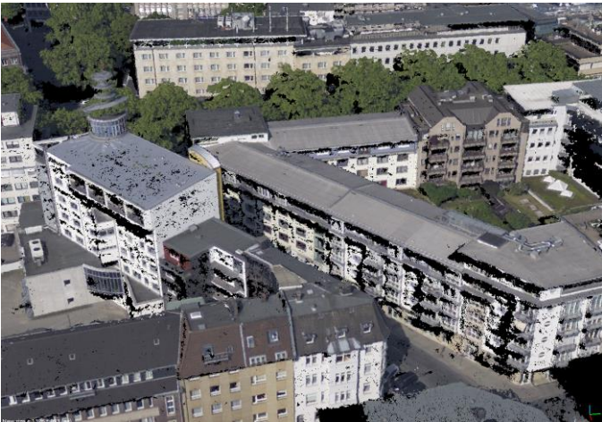
Fig. 7. 3D point cloud at building facades for complex urban area.
