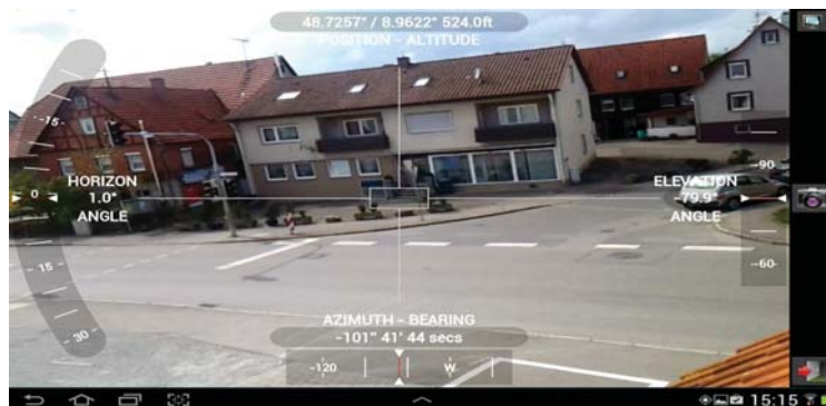
Figure 1. Mobile device screen to take pictures and additional pose information using AndroidSfM
