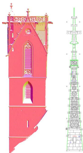
Figure 6: Left: Highlighting geometrical contours by color-coding normal vector directions (eastern facade). Right: Drawing of the south-western side of the tower helmet.
