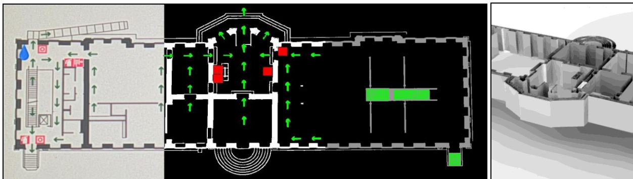
Figure 1. From left to right: pre-processed image; wall structures (white) and detected symbol areas (colored); symbol bridging edges and detected stair candidates (green); reconstructed 3D model
