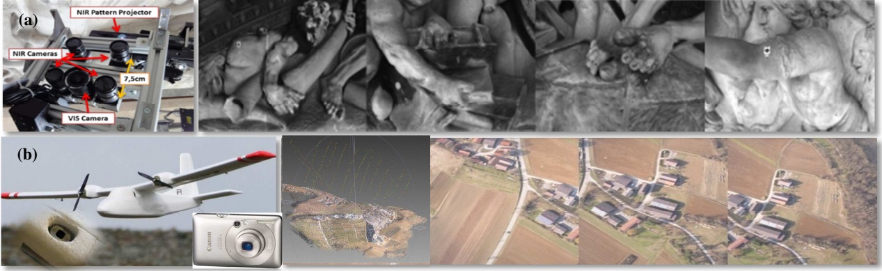
Figure 1: Low-cost sensors and its imagery. a) Five cameras rigidly mounted and protected by an aluminium frame. b) Fixed-wing UAV platform in flight, used consumer camera and mounting position on UAV belly. Right: Sparse point cloud and camera stations.
