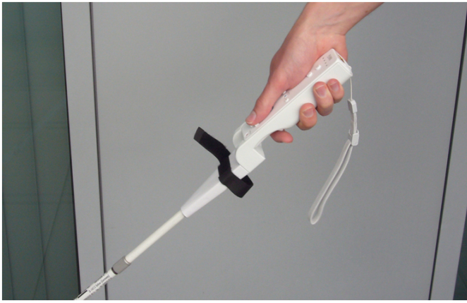
Fig. 5: The ViibraCane. In addition to direction guidance by vibration, the cane can be used as an input device to the navigation system.
