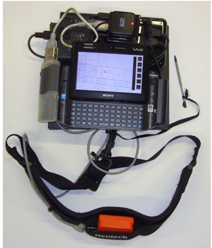
Fig. 4: The TANIA navigation system. The displayed map, acceleration sensor (on strap), rfid reader (left) and GPS receiver (top) can be seen.
