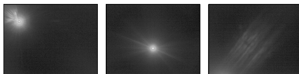
Fig. 2 Various stray light artefacts; left: fan, middle: beam, right: side light
