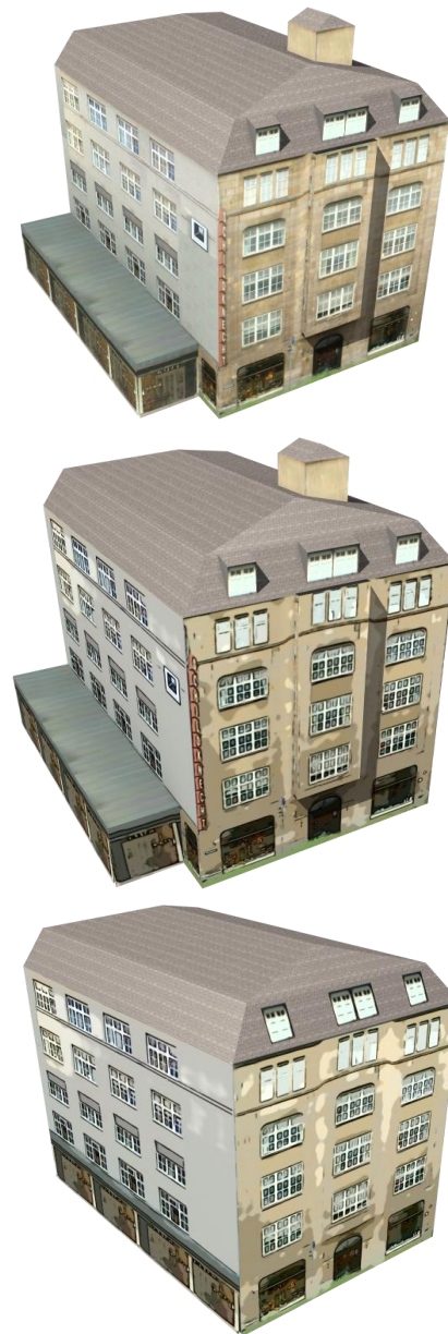
Figure 2: Two abstraction levels (1 st image, 2 nd geometry) from a photo-realistic 3D building model (top).
