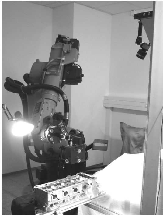
Fig. 1 Picture taken during a test at the University of Applied Sciences of Augsburg, which is one of our project partners. This successful joint experiment was performed in order to test data exchange between our camera system and the robot control unit.
