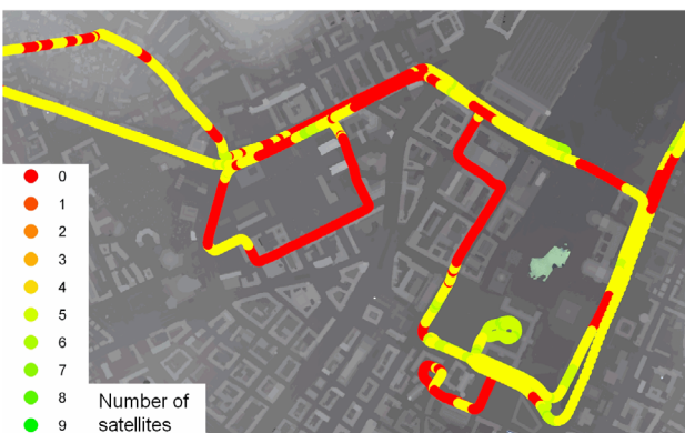
Figure 5 : Measured trajectory with number of visible satellites, overlaid to DSM of test area.
