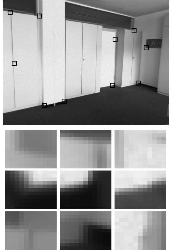
Figure 5. From the available feature points a fixed number of points are randomly selected for tracking, in this case ten are selected. The top figure shows the selected areas. The bottom figure is a composition of the image templates cut out in these areas.
