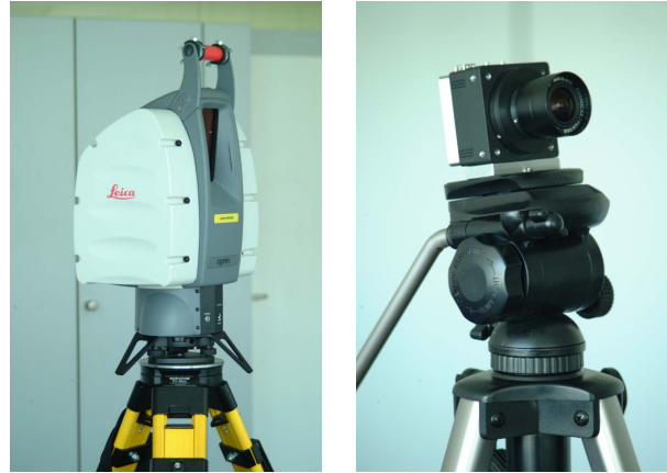
Figure 1. The sensors utilized for this study are a laser scanner and a machine vision camera. The laser scanner to the left is a Leica HDS 3000. The camera to the right is a Basler A302f. Both devices were mounted on a tripod during data acquisition.
