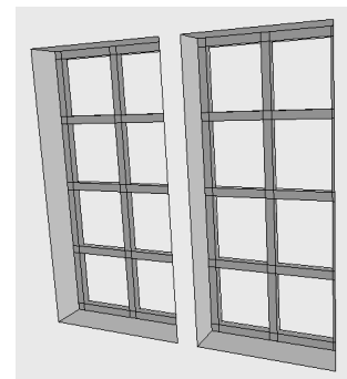
Figure 12. Reconstructed crossbars for two windows.
