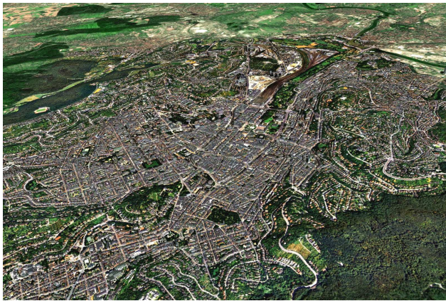
Figure 1. 3D real-time visualisation of the Stuttgart city model showing over 36,000 buildings (Kada et al, 2003)
