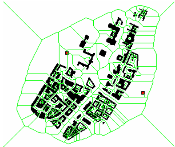
Figure 3. Calculation of the skeleton (in green colour) on a city map from Stuttgart. Start and end point: red square.
