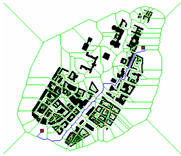
Figure 4. Calculation of the shortest path (in blue colour). Start end point: red square
