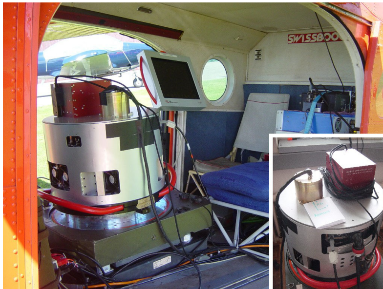
Figure 2: Aircraft installation ADS40 Vaihingen/Enz test flight (June 26, 2004).
