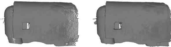
Figure 11: Difference of the first (left) and the third method (right) of splat radius computation shown on a detail of the dataset. By choosing larger splat sizes areas to the right with lesser density can still be adequately represented.
