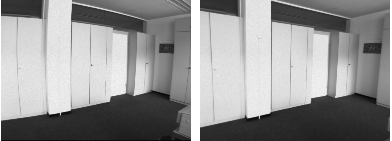
Figure 3. The lens distortion parameters and the coordinates of the principal point obtained during photogrammetric calibration are directly applied to the images. The left image shows an original frame from the sequence. The effects of lens distortions are particularly visible on the straight edges of the wall unit. The right image shows the processed image free of lens distortions.
