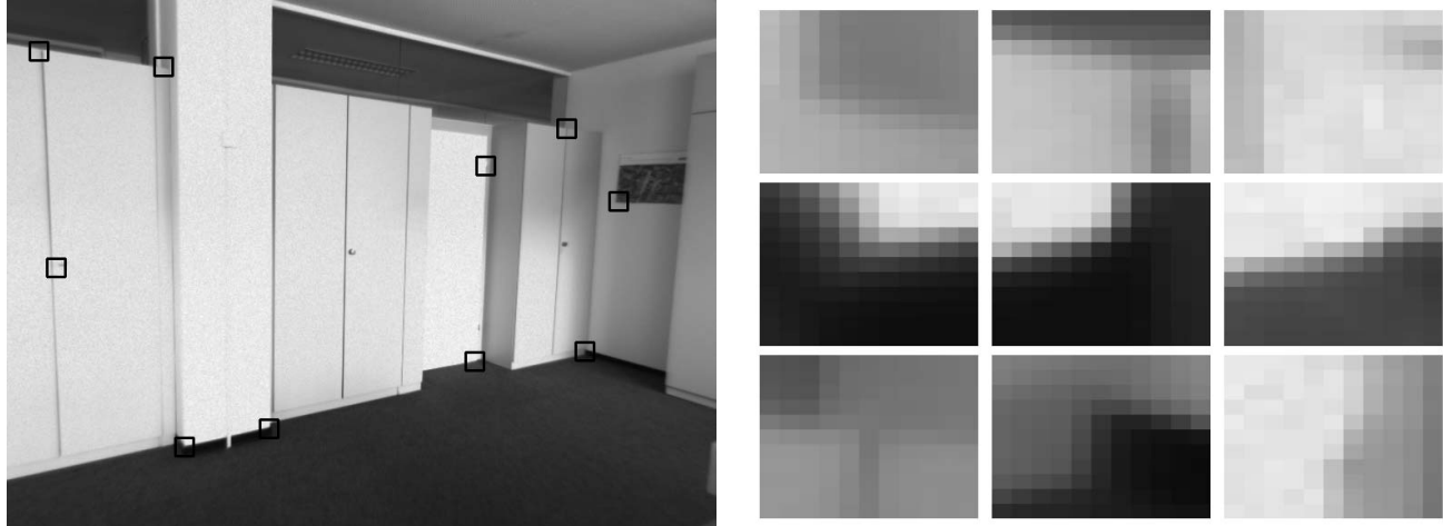
Figure 5. From the available feature points a fixed number of points are randomly selected for tracking, in this case ten are selected. The left figure shows the selected areas. The right figure is a composition of the image templates cut out in these areas.
