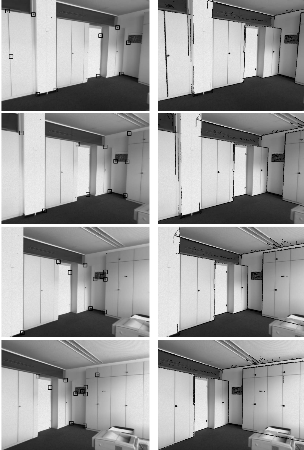
Figure 6. Four frames out of a sequence of 500 frames taken from an office environment. The four frames show a pan motion from left to right. The order of the sequence is from top to bottom. The left column shows the projected feature points, which were extracted from the laser range data. The features selected for tracking are marked with a box. The right columns shows the projection of the edge points extracted from the laser data onto the images.
