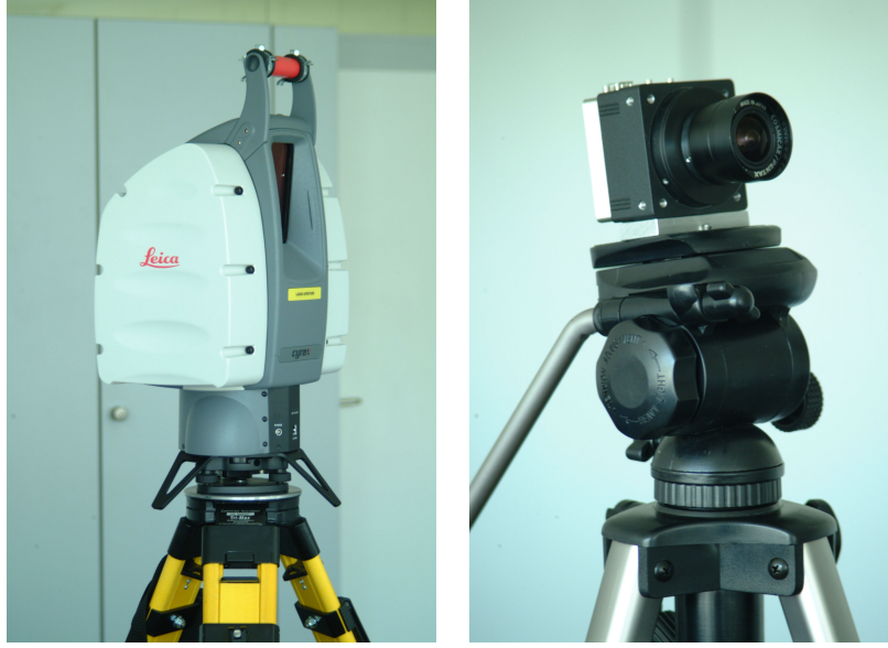
Figure 1. The sensors utilized for this study are a laser scanner and a machine vision camera. The laser scanner to the left is a Leica HDS 3000. The camera to the right is a Basler A302f. Both devices were mounted on a tripod during data acquisition.
