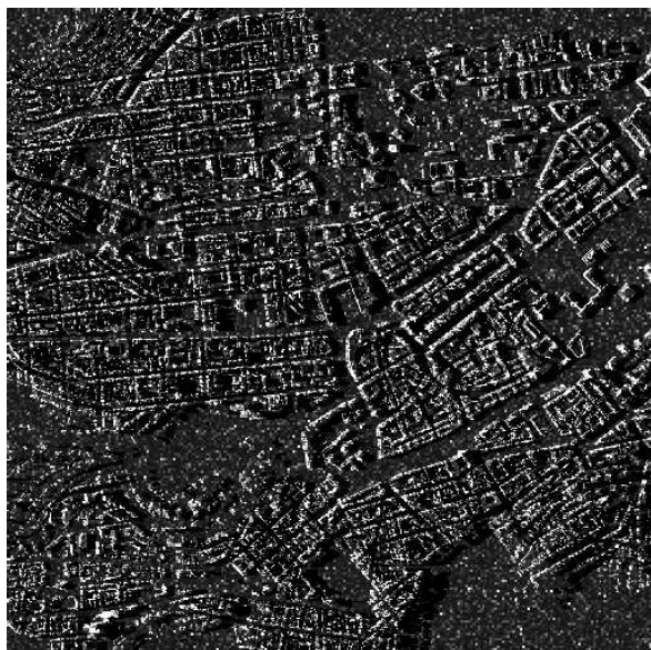
Figure 3. SARViz simulation of the 3D city model of Stuttgart (5m pixel resolution)
