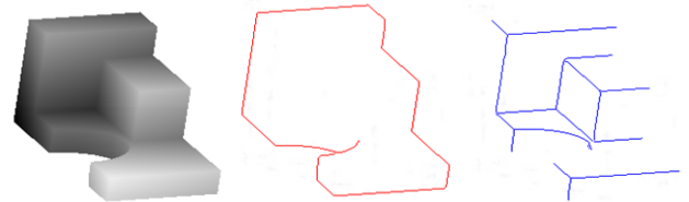
Figure 5. Curve block segmentation using different thresholds to detect step edges (red) and crease edges (blue).
