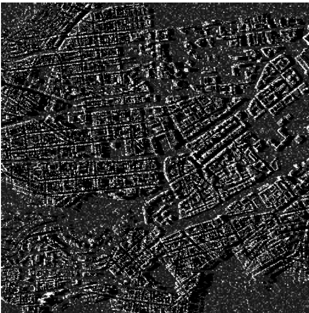
Figure 7. SARViz simulation of the 3D city model of Stuttgart (5m pixel resolution)
