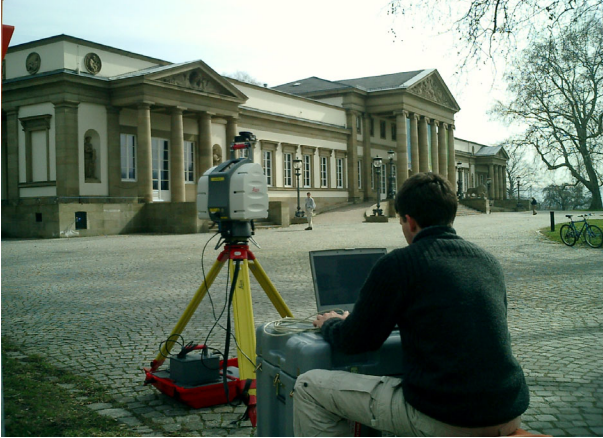
Figure 7. Terrestrial Laserscanning at Schloss Rosenstein.
