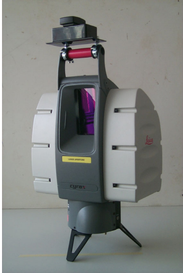
Figure 1. Laserscanner with low-cost GPS and digital compass.
