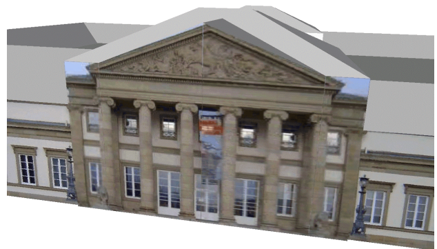
Figure 7: Resulting 3D building model with the extracted textures placed on the façade polygons.
