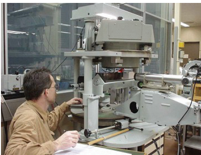
Figure 1: Goniometer at Zeiss Oberkochen (© Zeiss).
