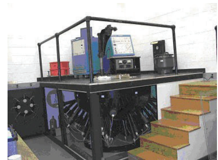
Figure 3: Multi-collimator at USGS OSL Reston (© USGS).
