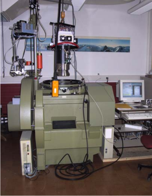
Figure 2, Gonimeter calibration of ADS40 at Leica (© Leica)
