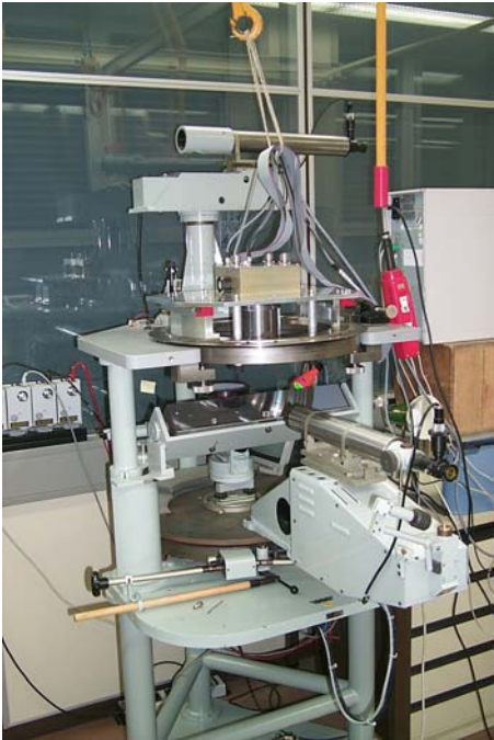
Figure 1, Gonimeter calibration of individual DMC camera head at Zeiss (© Zeiss)
