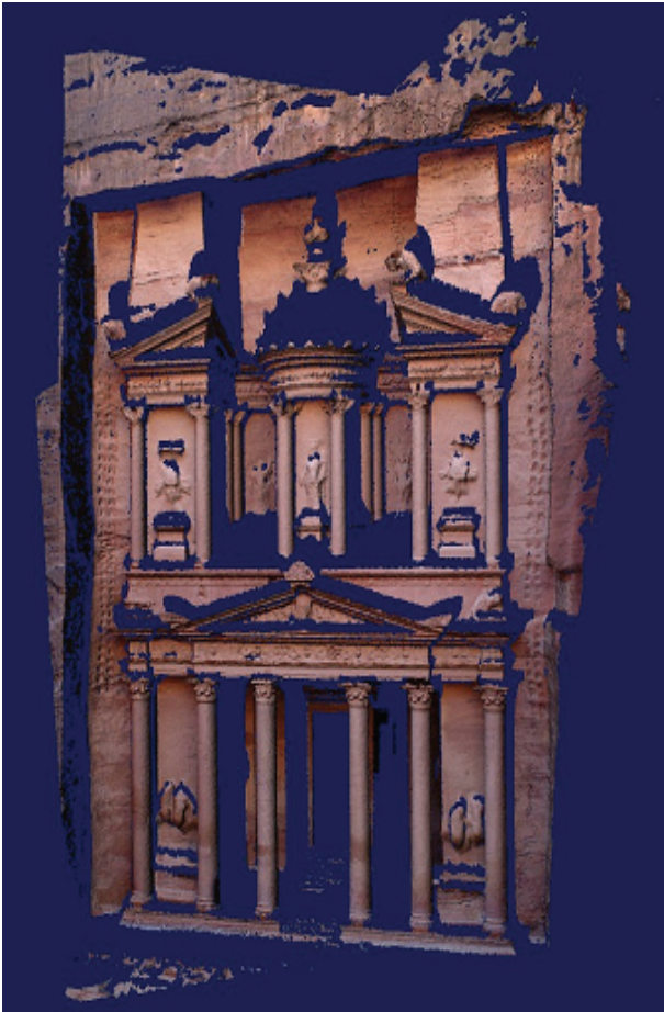
Figure 8. 3D textured model using master image after separating of the occluding parts
