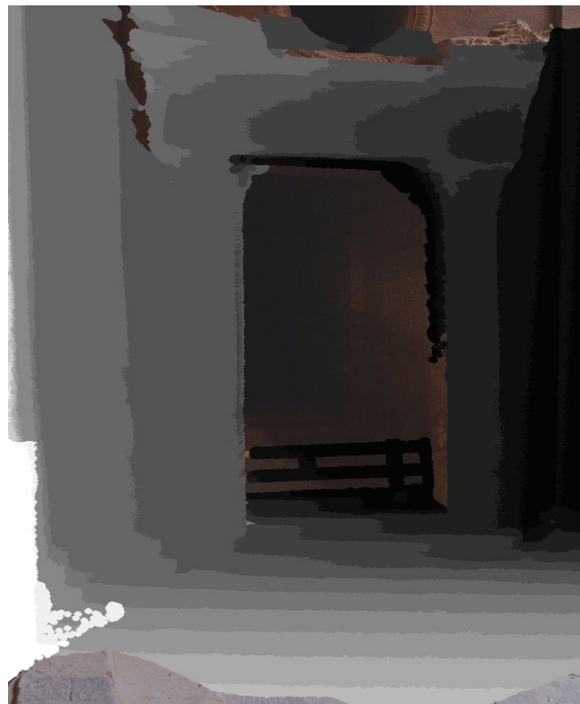
Figure 5. The distance image of the left door projected on the corresponding image.
