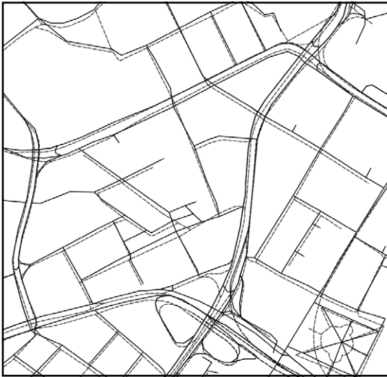
Figure 9. Clipping of the test scenario from the inner city of Stuttgart (ATKIS in dotted, GDF in straight lines).
