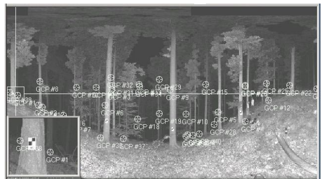
Figure 5: Measurement of corresponding points in panoramic (top) and reflectance image (bottom).
