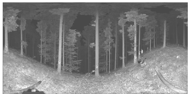
Figure 2: Reflectivity image captured from LIDAR scanner.
