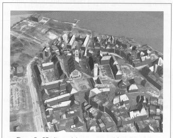
Figure 8. 3D city model reconstructed from lidar data.
