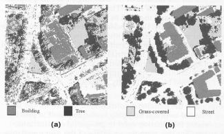
Figure 7. Improvement of classification results by integrating multispectral imagery and lidar data. (a) Channels: green, red, near infrared. (b) Channels: green, red, near infrared, normalized DSM. (Color version at www.asprs.org.)
