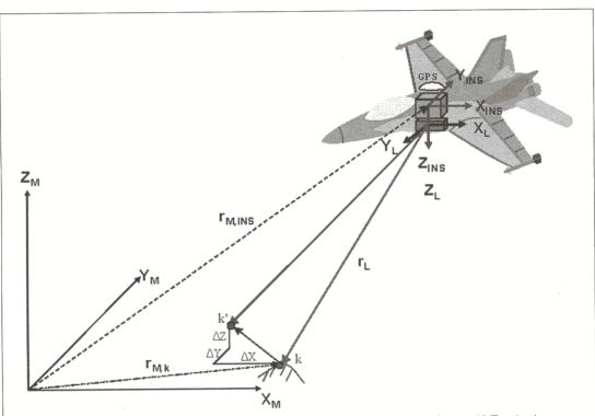
Figure 1. Lidar system sensor configuration:  $XYZ_L$  is the lidar reference frame,  $XYZ_{INS}$  is the INS body frame, and  $XYZ_M$  is the local mapping frame;  $\Delta X$ ,  $\Delta Y$ ,  $\Delta Z$  denote errors on the ground due to the boresight misalignment.
