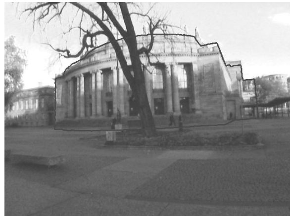
Figure 5: Image of the opera house with building silhouette overlaid. On the left the approximate orientation is used, on the right the result of the detection is displayed. Detection was successful despite the occlusions, shadowing effects and model imperfections.
