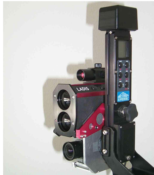
Figure 4: Prototype of the mobile photogrammetry device consisting of a camera, a compass and a tilt sensor. The GPS is mounted separately. The laser unit was not used in this project.
