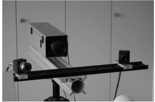
Figure 1: The sensor hardware used for the experiments consists of a LCD stripe projector and a digital camera.
