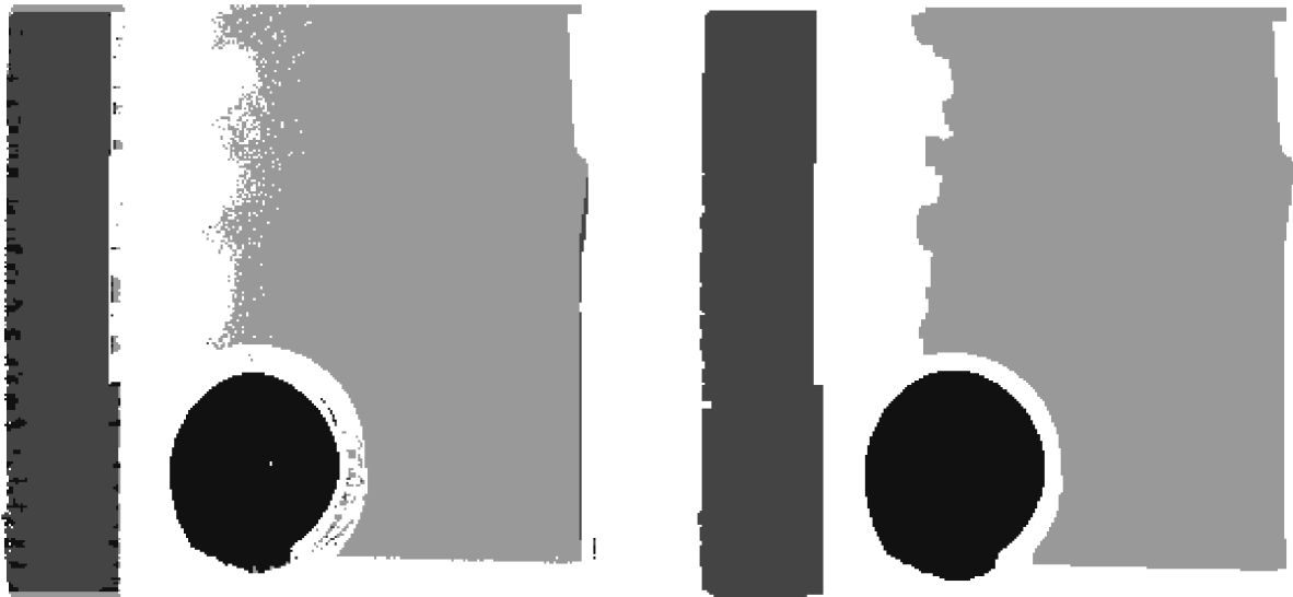
Figure 6: Segmentation results on the test scene. On the left the results after initial classification are shown. On the right the result after region growing and removal of sliver regions is shown.
