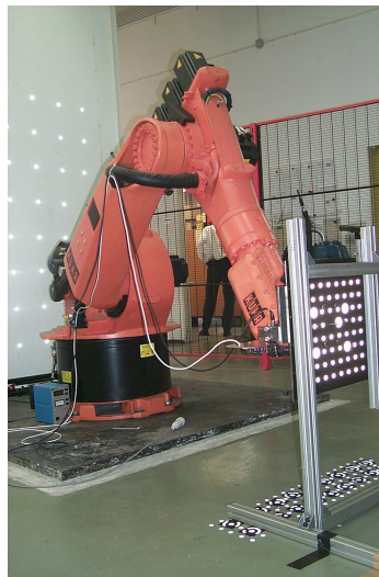
Figure 6: Robot with moving camera (at end effector) and stationary targets (on the ground).
