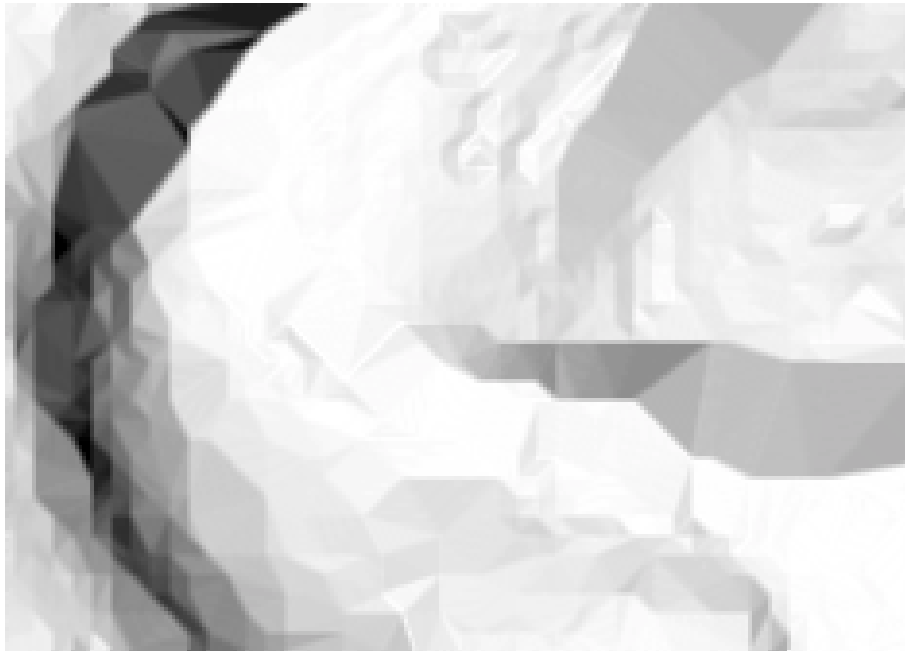
Figure 6: Uncertainty of the DTM data set given by variances of the heights. Variances are transformed into grey values (white = small variance, dark = large variance).
