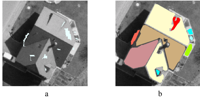
Figure 3: Region growing segmentation, a) extracted seed regions, and b) extracted 2-D plane-roof regions overlaid on corresponding building roof structure.
