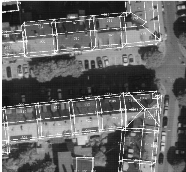
Figure 15: Reconstructed building projected into stereo image.
