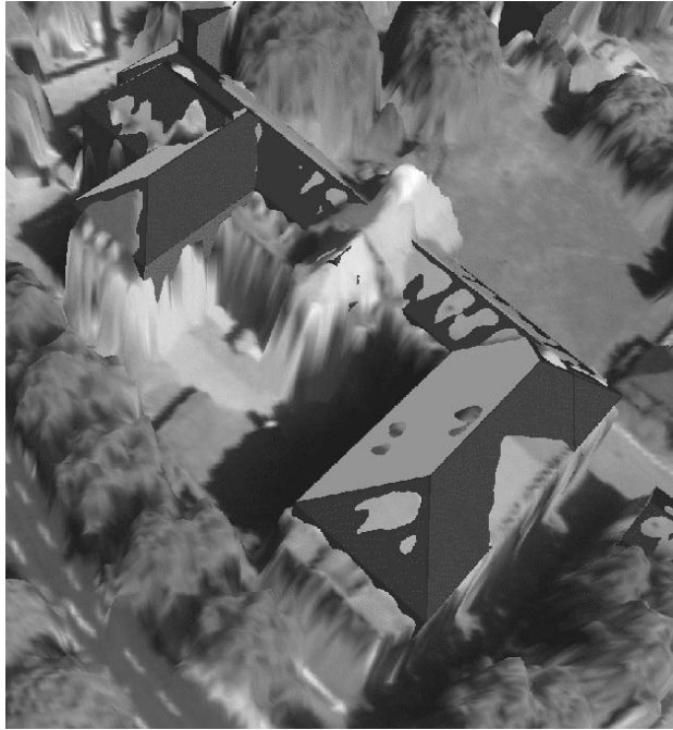
Figure 11: Automatically reconstructed building and DSM surface.
