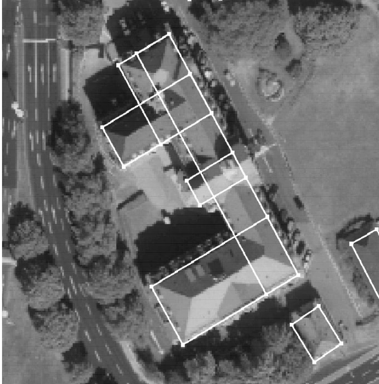
Figure 5: Ground plan decomposed into rectangular parts.
