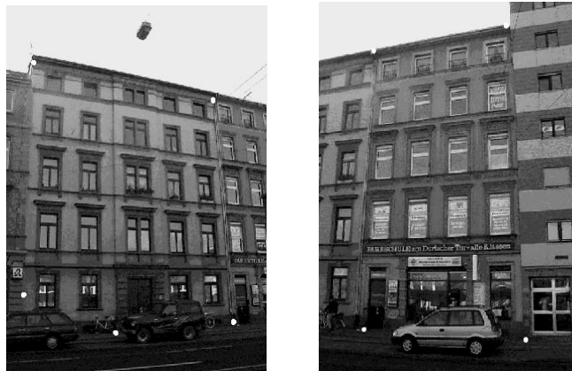
Figure 16: Original terrestrial images with points measured for rectification
