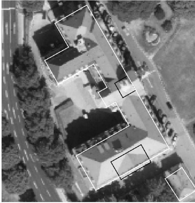
Figure 13: Building ground plan (white) an interactively added rectangles (black).
