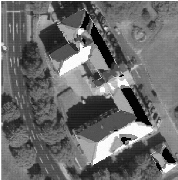
Figure 8: Original ground plan and segmented roof regions
