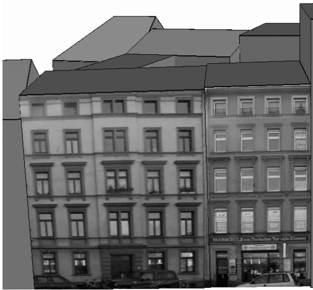
Figure 17: Faces mapped to corresponding 3D surfaces
